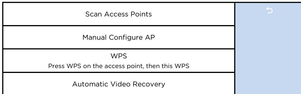
2. Press **Scan Access Points**. A list of available networks is displayed. Use the up and down arrows to scroll through the list. Press ↩ to return to the previous screen.
